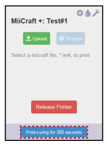
**2** The post curing starts and the UV lamp will automatically turn on.
